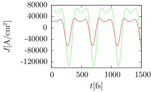
**Fig. 6.** (Color online) Time-dependent current density in  $\text{A}/\text{cm}^2$  as a function of time in fs for a frequency  $\omega = 0.01 \text{ eV}/\hbar$  and strength  $U_g = 0.1 \text{ eV}$  of the gate fields with phase difference  $\pi/2$  and  $\zeta/2\pi = 72.5 \text{ GHz}$ ,  $\gamma/2\pi = 24.2 \text{ THz}$  with self-consistent field (solid red line) and without self-consistent field (dashed green line).
