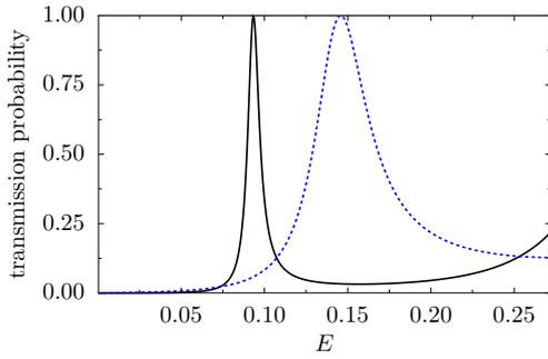
**Fig. 2.** (Color online) Tunneling transmission probability as a function of energy in eV for the static double barrier given in Fig. 1(b) (black line, see text for parameters) and its  $\delta$ -function approximation (dashed blue line) with  $V_{0,j} = 0.54$  a.u. and well width  $L = 7.345$  nm ( $= 141$  a.u.).
