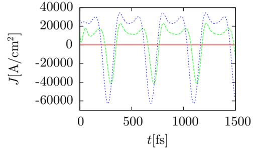
**Fig. 5.** (Color online) Time-dependent current density in A/cm<sup>2</sup> as a function of time in fs for three different values of the phase difference  $\varphi = 0$  (solid red line),  $\pi/4$  (long dashed green line),  $\pi/2$  (short dashed blue line) between the two gate fields with frequency  $\omega = 0.01$  eV/ $\hbar$  and strength  $U_g = 0.1$  eV and  $\zeta/2\pi = 72.5$  GHz,  $\gamma/2\pi = 24.2$  THz.
