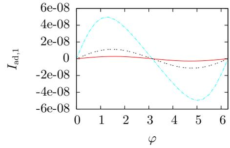
**Fig. 3.** (Color online) Adiabatic current  $I_{ad,1}$  in units of Ampère as a function of the difference between the phase of two gate fields for a driving frequency  $\omega = 4.13 \times 10^{12}$  Hz and different amplitudes  $V_{1,1} = 0.05$  a.u. (solid red line),  $V_{1,1} = 0.1$  a.u. (dashed black line),  $V_{1,1} = 0.2$  a.u. (turquoise dash-dotted line); additional parameters:  $V_{0,1} = V_{0,2} = 0.54$  a.u.,  $L = 7.35$  nm,  $m = 0.067 m_0$ ,  $\mu = 0.054$  eV,  $T = 300$  K.
