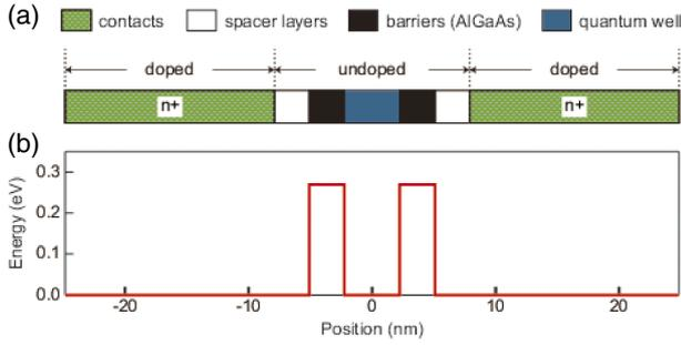
**Fig. 1.** (Color online) (a) Resonant tunneling structure with the quantum well of undoped GaAs and two barriers of undoped AlGaAs; spacer layers consist of undoped GaAs and contact regions of doped GaAs (doping concentration of  $2 \times 10^{18} \text{ cm}^{-3}$ ); (b) static double barrier potential.
