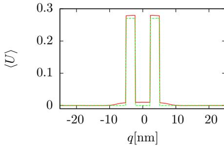
**Fig. 7.** (Color online) Average potential (in eV) for a frequency  $\omega = 0.01 \text{ eV}/\hbar$  and strength  $U_g = 0.1 \text{ eV}$  of the gate fields with phase difference  $\pi/2$  and  $\zeta/2\pi = 242 \text{ GHz}$ ,  $\gamma/2\pi = 24.2 \text{ THz}$  with self-consistent field (solid red line) and without self-consistent field (dashed green line).
